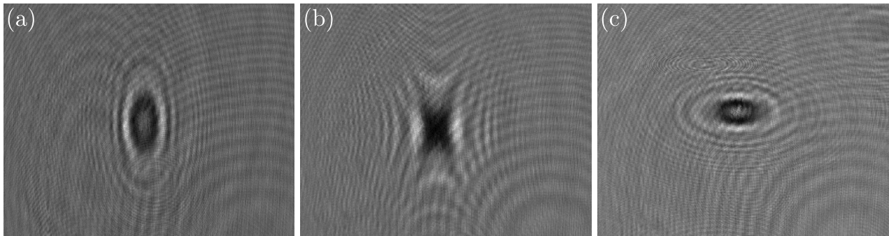
Fig. 2. Experimental acquisition of a 100 \mu\text{m} in diameter particle for (a) z_p \approx 55 mm, z \approx 165 mm ; (b) z_p \approx 80 mm, z \approx 140 mm ; z_p \approx 120 mm, z \approx 100 mm. Experimental parameters are roughly estimated by direct measurements on the set-up.
