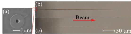
FIG. 4. (a) SEM image of the exit face (front surface) of the channel machined in fused silica using  $E = 8.6 \mu\text{J}/\text{pulse}$  and  $\tau_p = 4.7 \text{ ps}$ . (b) and (c) show OTM images (side-view) of the nanochannels before and after filling with water, respectively.
