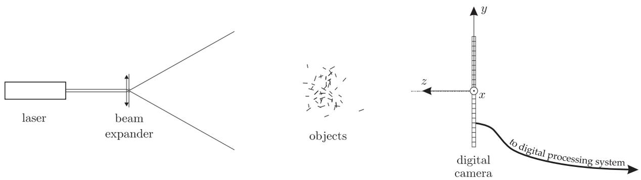
Fig. 1. Optical setup used in digital in-line holography
