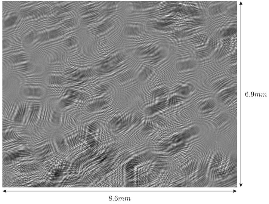
Fig. 10. Experimental hologram of paper fibers spread on a glass plate.
