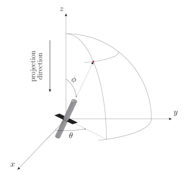
Fig. 2. Model of a short fiber and its orthogonal projection along the optical axis
