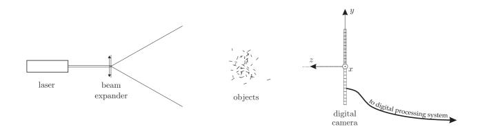
Fig. 1. Optical setup used in digital in-line holography
