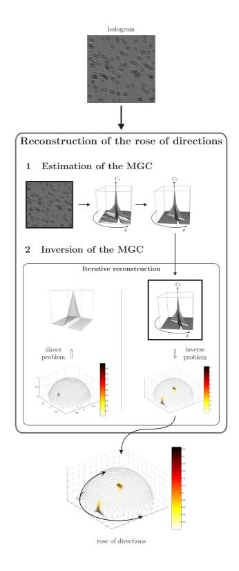
Fig. 5. Scheme of the method to reconstruct the rose of directions from an in-line hologram
