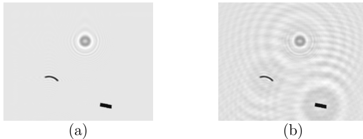
Figure 1. Twin-image appearing at the reconstruction step: (a) “twin-image free” reconstruction using the phase; (b) classical reconstruction from the hologram, showing the twin-image
