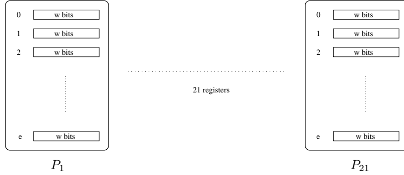
Figure 2: Memory Management of the ECM Unit
