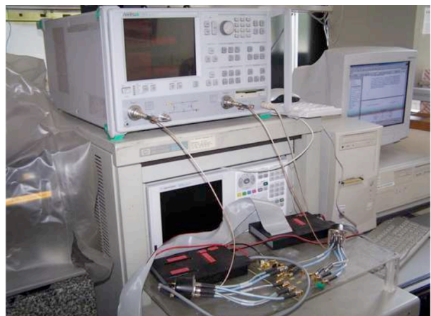
Figure 5 : Vector Network Analyzer used for the test CRL.
