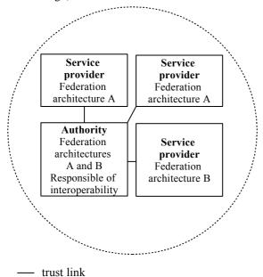
fig 1. Responsibility of interoperability in a federation architecture topology authority-centered with direct trust links.
