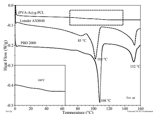
**Figure 7.** DSC thermograms of FAIMP exo-adduct in several polymer matrices 2<sup>nd</sup> heating cycle at 2°·min<sup>-1</sup>.
