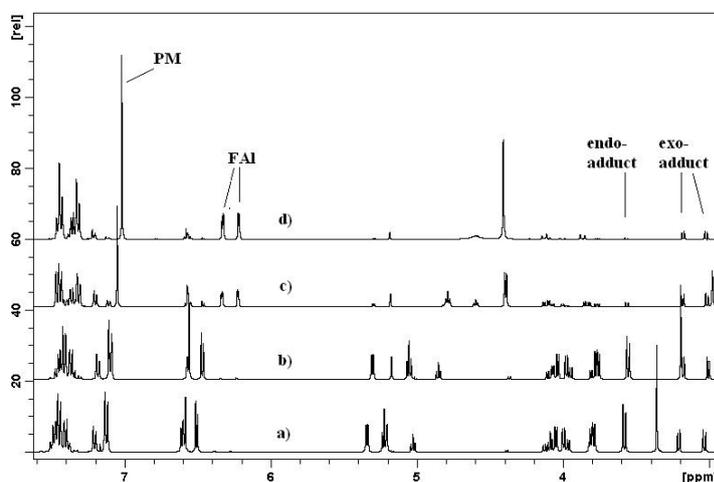
**Figure 1:** <sup>1</sup>H-NMR spectra of endo/exo-adduct in d<sub>6</sub>-DMSO at 25°C (a), 50°C (b), 90°C (c), 120°C (d).
