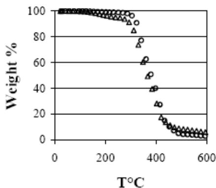
**Figure 10.** Dynamic thermogravimetric curves of (PVA-Ac)-g-PCL (○) and (PVA-Ac)-g-PCL/exo-adduct (△)
