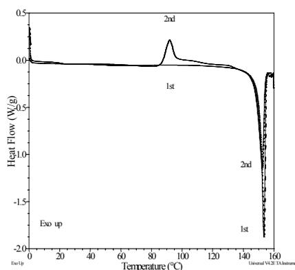
**Figure 3.** DSC thermograms of the exo-adduct heating cycles
