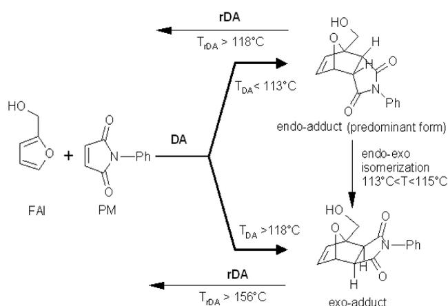
**Scheme 2.** DA and rDA reactions and isomerization of adducts.
