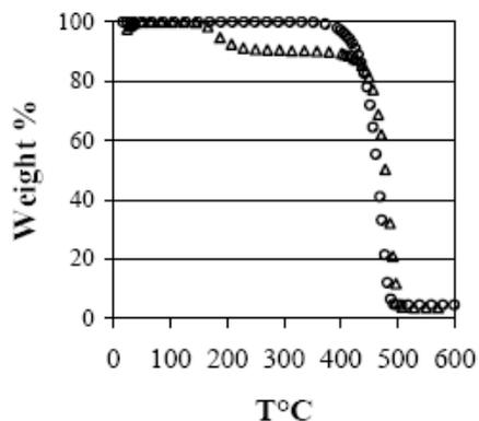
**Figure 8.** Dynamic thermogravimetric curves of PBD 2000 (○) and PBD 2000/exo-adduct (△)
