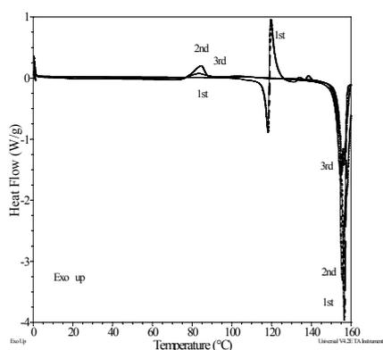
**Figure 2.** DSC thermograms of the endo/exo-adduct heating cycles
