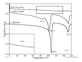
**Figure 7.** DSC thermograms of FAIMP exo-adduct in several polymer matrices  $2^{\text{nd}}$  heating cycle at  $2^{\circ}$ .min<sup>-1</sup>.
