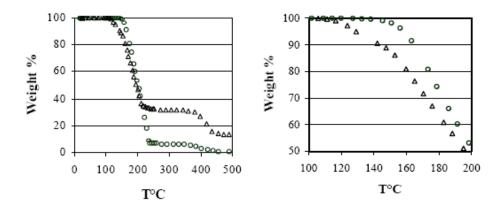
**Figure 6a.** Dynamic thermogravimetric curves for exo-adduct ( $\circ$ ) and endo/exo-adduct ( $\triangle$ ) Figure 6b. view of Figure 6a between 100°C and 200°C
