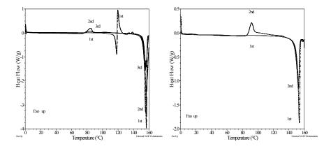
**Figure 2**. DSC thermograms of the endo/exo-adduct heating cycles
