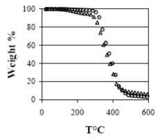
Figure 10. Dynamic thermogravimetric curves of (PVA-Ac)-g-PCL (o) and (PVA-Ac)-g-PCL/exo-adduct ( $\triangle$ )
