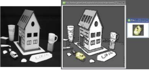
Figure 5. Finding a car in an image: The original image, coming from the MOVI dataset (Luo et al., 2003), is on the left. The plane graph obtained after segmentation is on the middle. The car has been extracted and rotated on the right. It is found again in the original image using Damiand et al.(2009)’s algorithm.
