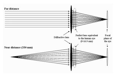
Fig. 3. Optical system used in the simulation of the MTF with Zemax® for near and far objects.
