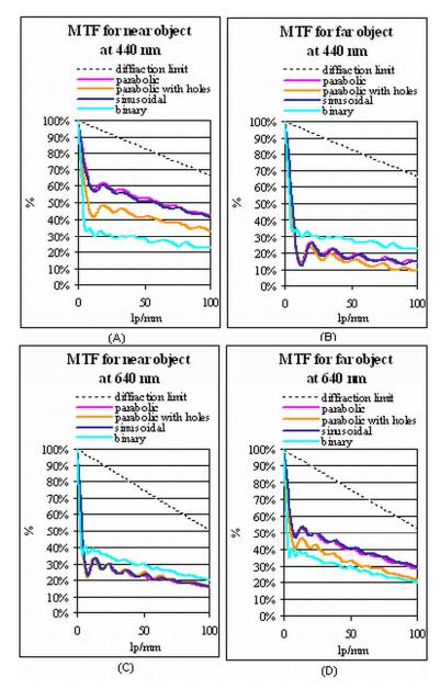
Fig. 6. MTFs for the near and far vision, at 440 nm and 640 nm.
