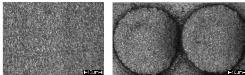
**Fig. 6.** Optical microscope image X2000 of ripples obtained with the “optical way 2” femtosecond laser chain (25 mW, 0.4 J.cm<sup>-2</sup>, 150 fs, 800 nm, 5 kHz, achromat doublet lenses: f = 50.8 mm). The overlapping process is use on the left, and the point by point process is used on the right.
