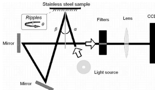
**Fig. 3.** Schematic Illustration of the light's optical path in a used scanner showed the principle of the reading procedure (see text).
