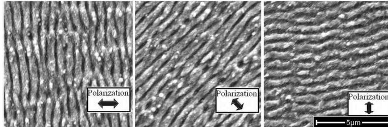
**Fig. 7.** SEM image X6000 of ripples obtained with the “optical way 2” femtosecond laser chain ( $P = 100 \text{ mW}$ ,  $F = 1.6 \text{ J.cm}^{-2}$ , rotating mirrors speed =  $20 \text{ mm.s}^{-1}$ ) on stainless steel 316L. On the left, ripples marked with a  $0^\circ$  polarization angle. In middle, ripples marked with a  $45^\circ$  polarization angle. On the right, ripples marked with a  $90^\circ$  polarization angle.
