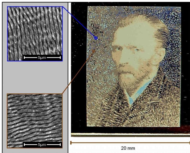
**Fig. 1.** On the right, example of color effects obtained by controlled nanostructures with a femtosecond laser chain on a 316L stainless steel sample, on the left, SEM X6000 images of controlled nanostructures marked with two different orientations.
