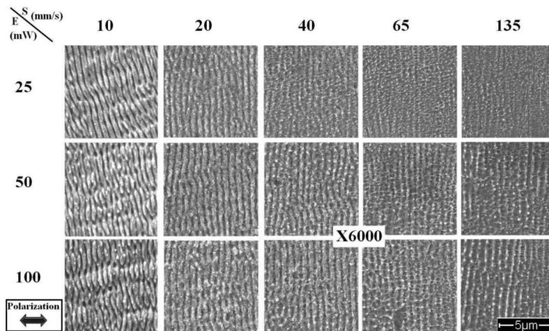
**Fig. 4.** SEM X6000 images of ripples obtained with the “optical way 2” femtosecond laser chain (150 fs, 800 nm, 5 kHz, achromat doublet lenses:  $f = 50.8$  mm) on stainless steel 316L. The different ripples aspects are obtained with a beam power from 25 mW to 100 mW (fluence from 0.4 J.cm<sup>-2</sup> to 1.6 J.cm<sup>-2</sup>) for rotating mirrors speed from 20 mm.s<sup>-1</sup> to 130 mm.s<sup>-1</sup>.
