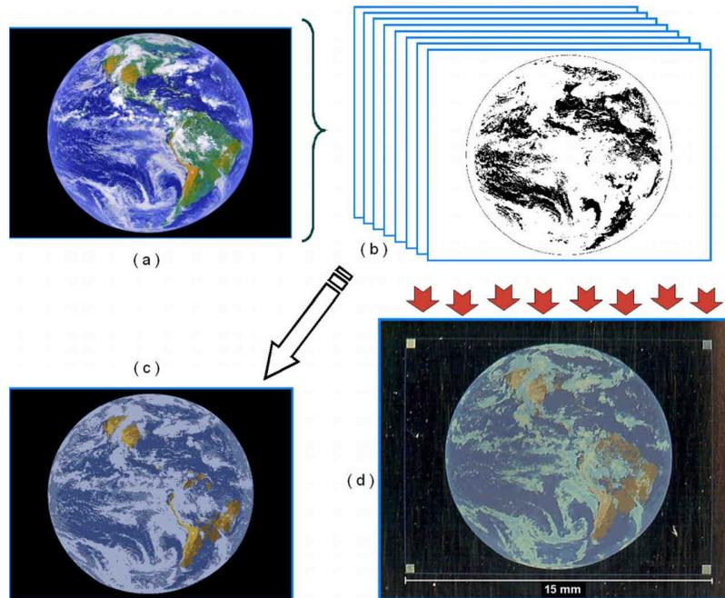
**Fig. 12.** Segmentation by image processing into height laser marking planes (b) of an initial image (a) and computer simulation of the expected color marking result (c). Scanner image (1200 dpi) of stainless steel sample (316L) marked with height planes of ripples (d). Each plane is marked with his own ripples orientation.
