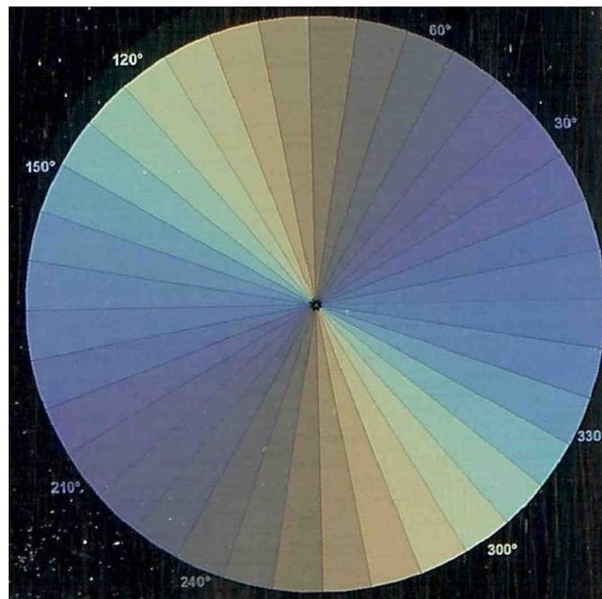
**Fig. 9.** Scanned image (1200 dpi) of stainless steel sample (316L) marked by thirty six discs section obtained with the “optical way 1” femtosecond laser chain ( $P = 25 \text{ mW}$ ,  $F = 0.4 \text{ J.cm}^{-2}$ ). Each section have been marked with different ripples orientations (from  $0^\circ$  to  $350^\circ$ ).
