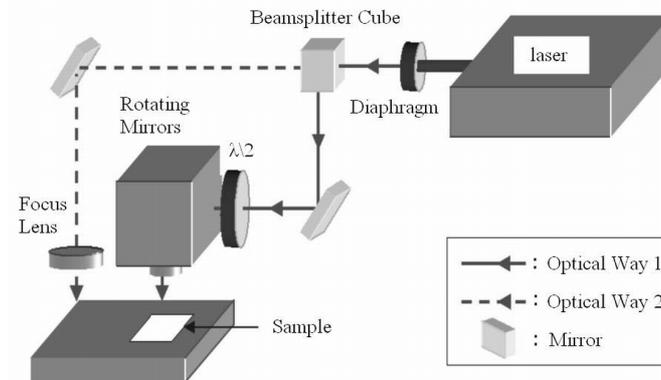
**Fig. 2.** Writing experimental set up with a femtosecond laser ( 2 W, 150 fs, 800 nm, 5 kHz). The figure show the two optical ways use in this article. The optical way 1 uses a rotating mirrors (HurrySCAN) with a F-Theta objective lens ( $f = 88$  mm) and the optical way 2 uses an achromat doublet lenses ( $f = 50.8$  mm).
