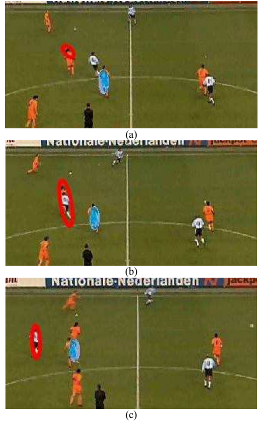
Figure 6 (a) The object is tracked at frame 54 (b) The object is almost fully occluded at frame 57 (c)Track wrong object at frame 62
