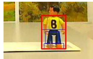
Figure 2 Maximum rectangle (thick red) of body, trouser and shoes' rectangle (thin blue).
