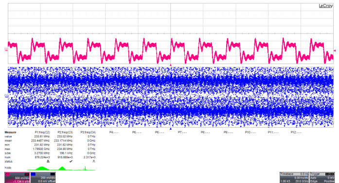
Fig. 6. Unlocked ring oscillators. Trigger on top signal.
