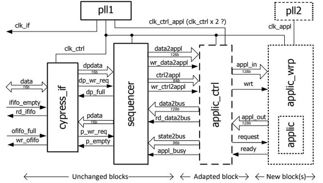
Fig. 4. Typical top level VHDL entity structure
