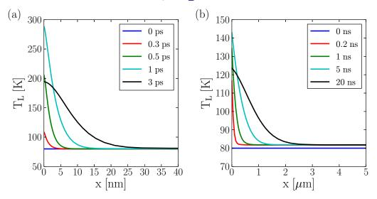
**Figure 2.** Spatial distributions of lattice temperature for a Ge sample at different times (a) with dc field  $E_0 = 1.5 \text{ V nm}^{-1}$  and (b) without dc field x = 0 corresponds to the surface of the sample. The surface recombination velocity is  $v_{\rm sr} = 10^6 \text{ cm s}^{-1}$ . Laser pulse parameters:  $I = 1 \text{ GW cm}^{-2}$ ,  $\tau_{\rm p} = 500 \text{ fs}$ , the pulse peak at 600 fs.
