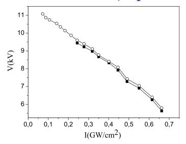
**Figure 5.** The dc voltage as a function of the laser intensity at  $2 \times 10^{-3}$  detected atoms per pulse for a tungsten tip. Full squares correspond to the data collected for a base temperature of 80 K and open dots correspond to a base temperature of 20 K.
