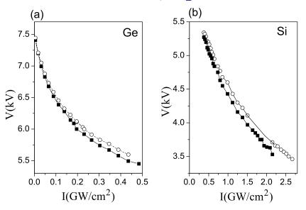
**Figure 6.** The dc voltage as a function of the laser intensity at  $2 \times 10^{-3}$  detected atoms per pulse for (a) the Ge tip and (b) the Si tip. Full squares correspond to the data collected for a base temperature of 80 K and open dots correspond to a base temperature of 20 K.
