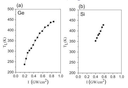
**Figure 8.** Temperature of the tip as a function of the laser intensity for a fixed voltage V. (a) the Ge tip, V = 5.5 kV; (b) the Si tip, V = 5 kV.
