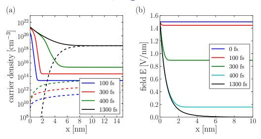
**Figure 1.** Spatial profiles inside the Ge sample at different times for (a) hole density (solid lines) and electron density (dashed lines) and (b) dc electric field. x = 0 corresponds to the surface of the sample. Laser pulse parameters:  $I = 1 \text{ GW cm}^{-2}$ ,  $\tau_p = 500 \text{ fs}$ , the pulse peak at 600 fs. The external dc field at the surface  $E_0 = 1.5 \text{ V nm}^{-1}$ . The surface recombination velocity  $v_{sr} = 10^6 \text{ cm s}^{-1}$ .
