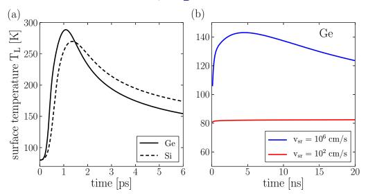
**Figure 3.** Lattice temperature at the surface  $T_L(x = 0)$  as a function of time (a) with a dc field  $E_0 = 1.5 \text{ V m}^{-1}$  for the Ge sample and  $E_0 = 2 \text{ V m}^{-1}$  for Si; (b) without a dc field for the Ge sample for different values of surface recombination velocity  $v_{sr}$ .
