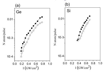
**Figure 7.** The number of detected atoms per pulse as a function of laser intensity for (a) the Ge tip and (b) the Si tip. Full squares correspond to the data collected for a base temperature of 80 K and open dots correspond to a base temperature of 20 K.
