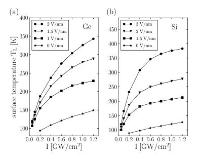
**Figure 4.** Surface peak temperature of Ge (a) and Si (b) samples as a function of laser pulse intensity at different values of dc field  $E_0$ . Pulse width  $\tau_p = 500$  fs and the surface recombination velocity  $v_{sr} = 10^6$  cm s<sup>-1</sup>.
