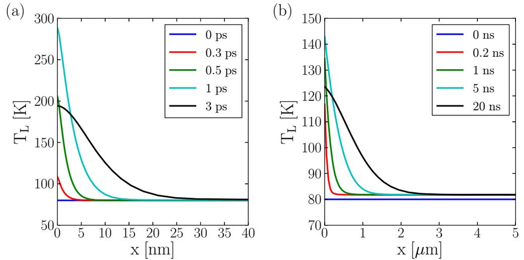
**Figure 2.** Spatial distributions of lattice temperature for a Ge sample at different times (a) with dc field  $E_0 = 1.5 \text{ V nm}^{-1}$  and (b) without dc field  $x = 0$  corresponds to the surface of the sample. The surface recombination velocity is  $v_{\text{sr}} = 10^6 \text{ cm s}^{-1}$ . Laser pulse parameters:  $I = 1 \text{ GW cm}^{-2}$ ,  $\tau_p = 500 \text{ fs}$ , the pulse peak at 600 fs.
