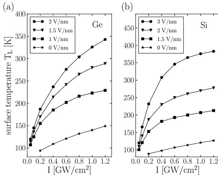
**Figure 4.** Surface peak temperature of Ge (a) and Si (b) samples as a function of laser pulse intensity at different values of dc field  $E_0$ . Pulse width  $\tau_p = 500 \text{ fs}$  and the surface recombination velocity  $v_{sr} = 10^6 \text{ cm s}^{-1}$ .
