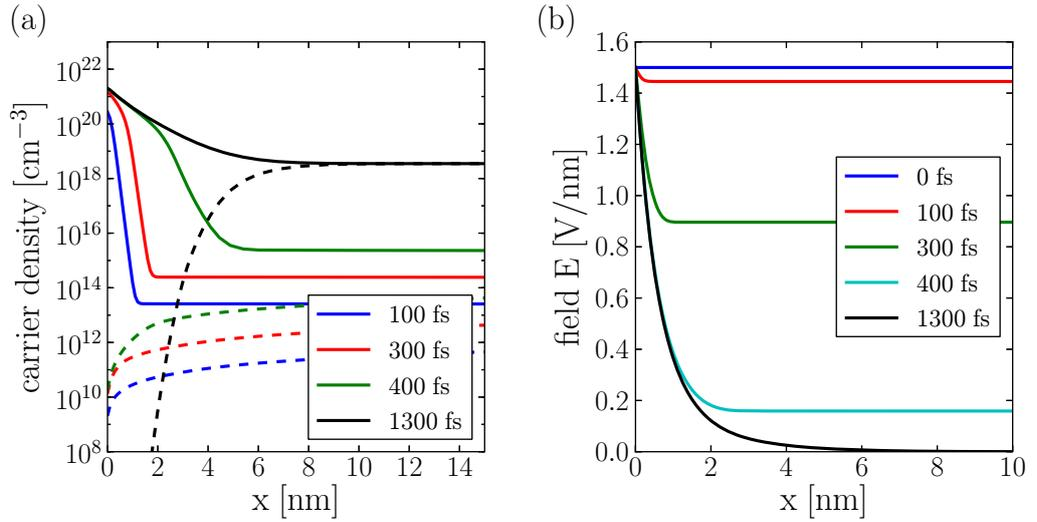
**Figure 1.** Spatial profiles inside the Ge sample at different times for (a) hole density (solid lines) and electron density (dashed lines) and (b) dc electric field.  $x = 0$  corresponds to the surface of the sample. Laser pulse parameters:  $I = 1 \text{ GW cm}^{-2}$ ,  $\tau_p = 500 \text{ fs}$ , the pulse peak at 600 fs. The external dc field at the surface  $E_0 = 1.5 \text{ V nm}^{-1}$ . The surface recombination velocity  $v_{sr} = 10^6 \text{ cm s}^{-1}$ .
