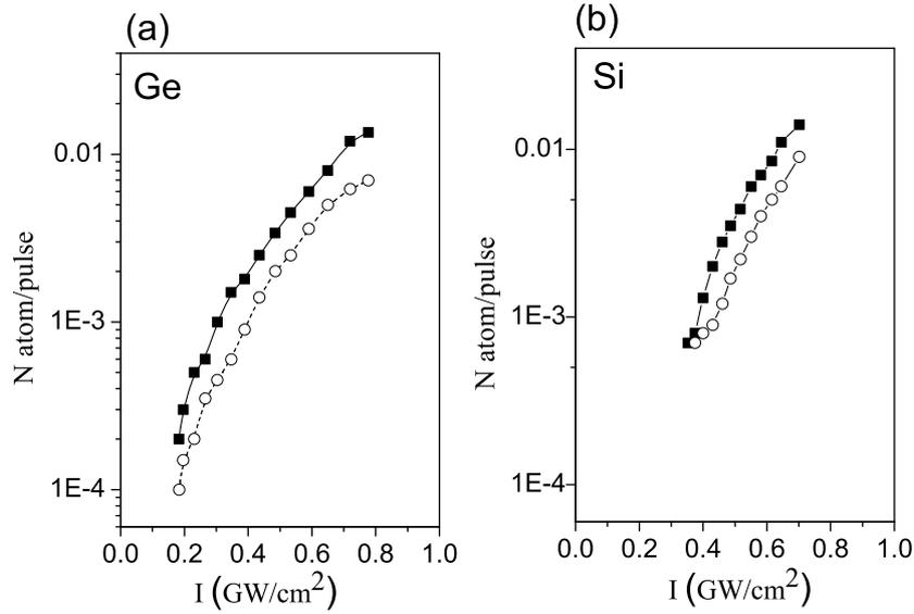
**Figure 7.** The number of detected atoms per pulse as a function of laser intensity for (a) the Ge tip and (b) the Si tip. Full squares correspond to the data collected for a base temperature of 80 K and open dots correspond to a base temperature of 20 K.
