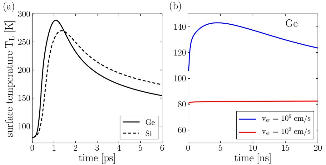
**Figure 3.** Lattice temperature at the surface  $T_L(x = 0)$  as a function of time (a) with a dc field  $E_0 = 1.5 \text{ V m}^{-1}$  for the Ge sample and  $E_0 = 2 \text{ V nm}^{-1}$  for Si; (b) without a dc field for the Ge sample for different values of surface recombination velocity  $v_{sr}$ .
