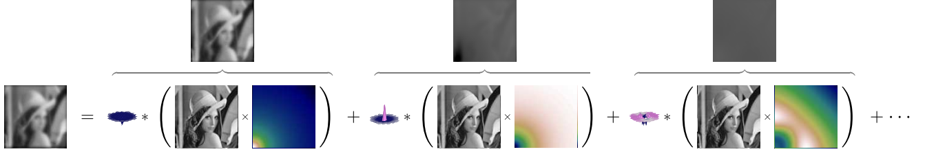
(c) interpolation of PSF: shown to be equivalent to the approach of Hirsch et al. (2010)
