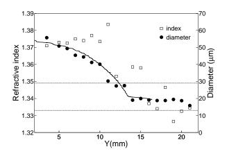
Fig. 9 Refractive index and diameter of a droplet measured at rainbow angle as a function of its distance from the injector. - diameter evolution of a droplet of the same size as measured at a different time by holography.
