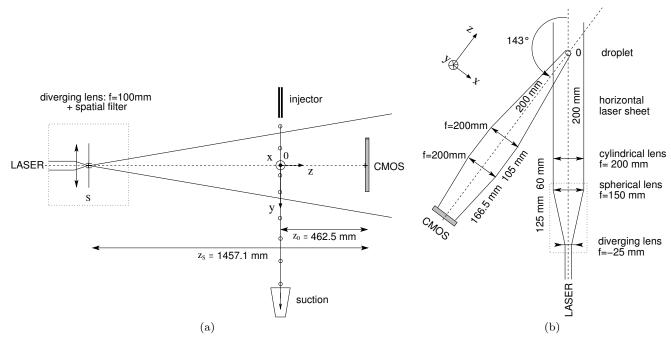
Fig. 1 (a) Holographic and injection setup. (b) Rainbow measurements setup.
