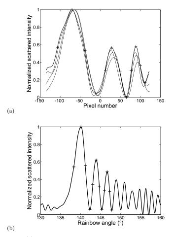
Fig. 6 (a): Patterns of Fig. 5 after filtering; the correspondence between pixel number and scattering angle for the pattern in bold is achieved with the characteristics points represented by the crosses. (b) Filtered theoretical pattern calculated with LMT for a 65.8  $\mu$ m diameter water droplet.
