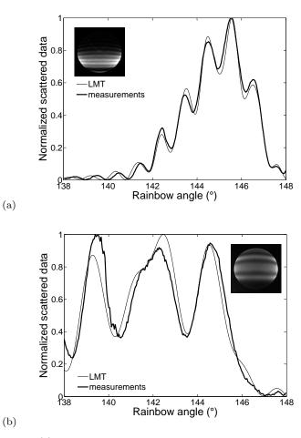
**Fig. 8** (a): The best fit between LMT and measurements is obtained for n= 1.3725 and d= 49.3428  $\mu$ m; the droplet is located at Y= 6 mm from the injector (see Fig.9). (b): The best fit between LMT and measurements is obtained for n= 1.3375 and d= 19.1070  $\mu$ m; the droplet is located at Y= 16 mm from the injector.
