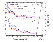
Figure 5:  $T_e$  dependent optical indices of  $\gamma$ -Fe, real part in a) and imaginary part in b). The experimental data of  $\alpha$ -Fe is also provided in black dots. <sup>48,49</sup> c) the thermal conductivity (K<sub>th</sub>), exhibiting a strong dependency on the electronic temperature.
