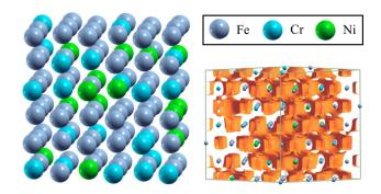
Figure 1: The 108 atoms supercell of 316L stainless steel generated with the SQS method (left), and a representation of the electronic density at  $T_e = 4 \times 10^4$  K (right).
