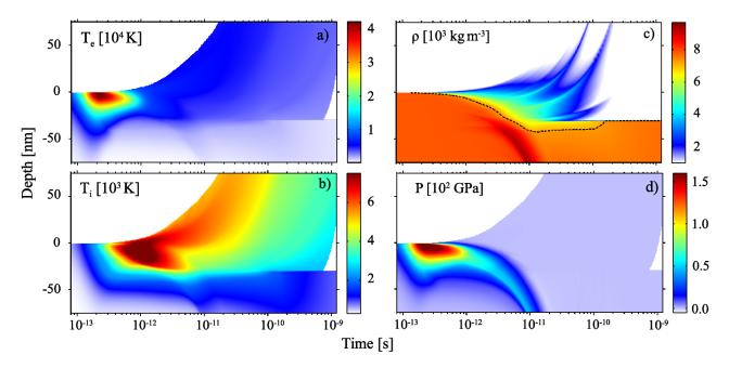
Figure 6: Spatio-temporal evolution of a) electronic temperature, b) matter temperature, c) material density and d) total pressure in a hydrodynamic simulation of a 316L stainless steel target irradiated with a 100 fs laser pulse at an incident fluence of 0.6 Jcm<sup>-2</sup>. Simulation parameters integrate nonequilibrium electronic data presented in previous sections.
