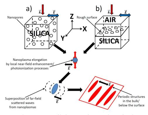
**Figure 1.** Schematic representation of the electromagnetic formation mechanisms of periodic nanostructures for (**a**) bulk and (**b**) surface ultrashort laser nanoprocessing.
