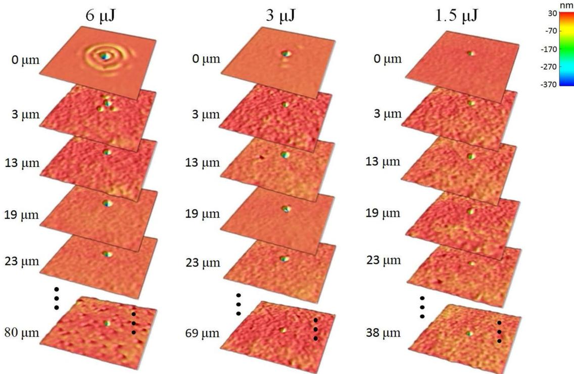
**Fig. 4** Tomography of channels is revealed by layer-by-layer polishing and surface imaging with confocal microscopy in 6, 3, and 1.5  $\mu\text{J}$  cases. All layer images have the size of  $14 \times 14 \mu\text{m}^2$ . The depth
