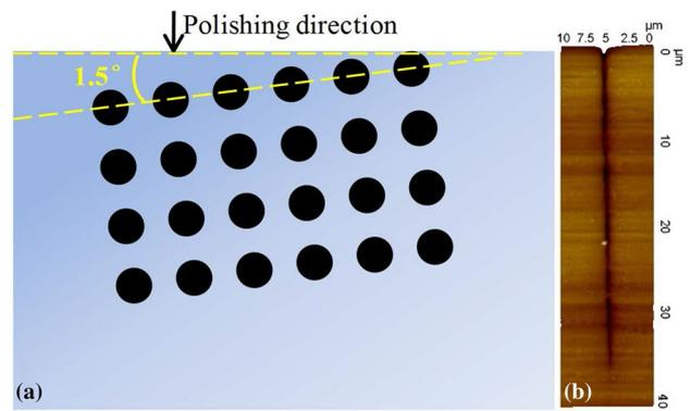
**Fig. 3** **a** Scheme of principle for successful application of post-polishing procedure: an array of channels is fabricated to enhance the hitting possibility to expose the axial profile of channels during the polishing procedure. **b** Partially exposed longitudinal section of channel (3  $\mu\text{J}$  case) is characterized by AFM
