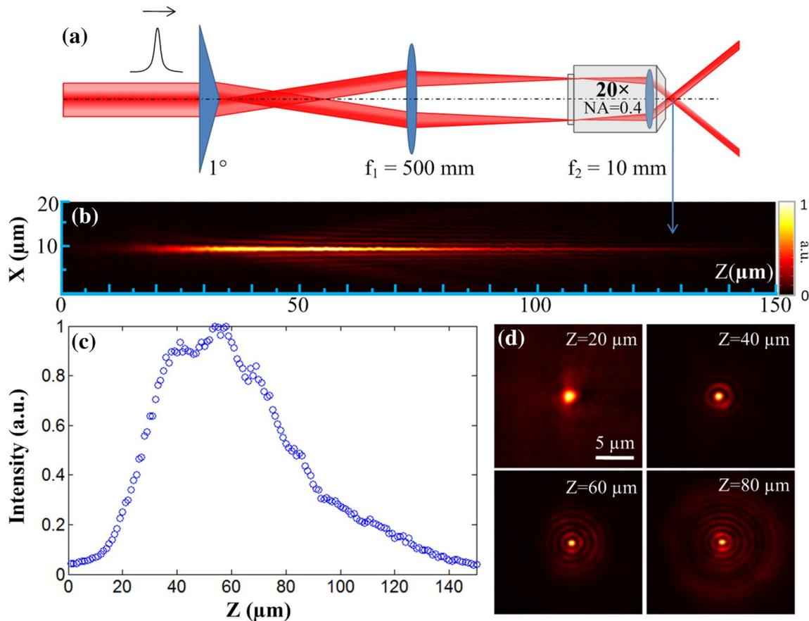
**Fig. 1** Characterization of the Gaussian–Bessel beam in the air. **a** Schematic diagram of 4-f setup for generating the desired beam. **b** Reconstructed beam intensity profile along the optical axis. **c** Beam
