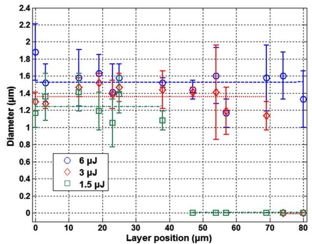
**Fig. 5** Diameter of channel versus layer position and for different pulse energy cases (6, 3, and 1.5  $\mu\text{J}$ ). Data are extracted from tomography measurement in Fig. 4 and the diameter is estimated as the average size of the orthogonal directions. The dashed lines are added to guide the eye
