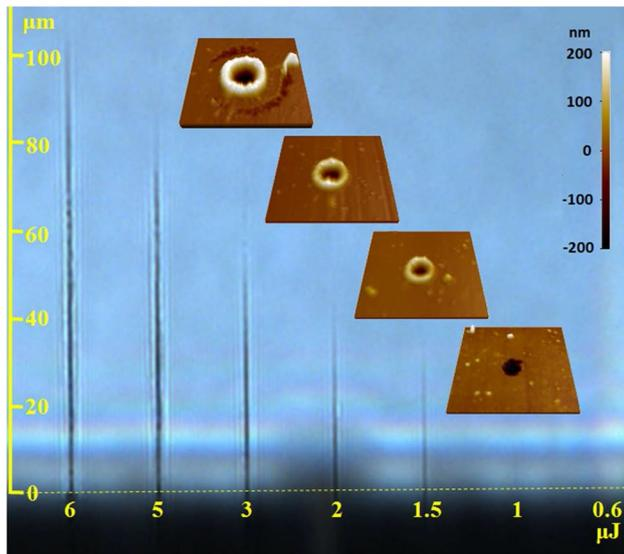
**Fig. 2** Transmission optical microscope reveals the evolution of bulk modification as a function of the pulse energy (from 6 to 0.6  $\mu\text{J}$ ). Laser beam comes from the bottom of the image. The insets ( $5 \times 5 \mu\text{m}^2$ ) on the top of the channels are the corresponding surface morphologies (from 3 to 1  $\mu\text{J}$ ) characterized by atomic force microscopy (AFM, PSIA XE-100). Scale bar describing the vertical axis is added for reference
