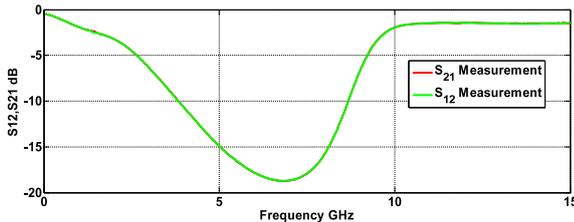
**Fig. 6.** Transmission  $S$ -parameters in the demagnetized state.
