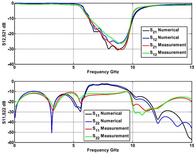
**Fig. 4.**  $S$ -parameters: comparison of the measured  $S$ -parameters and the  $S$ -parameters calculated using the optimization process (transmission parameters and reflection parameters) with an applied magnetic field of  $H_0 = 178$  kA/m.
