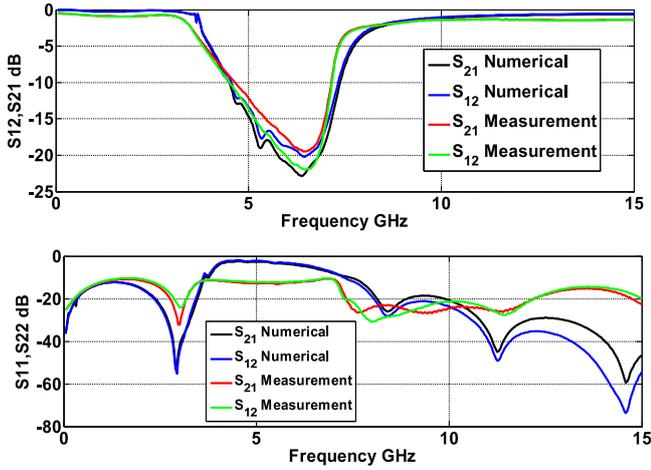
**Fig. 3.**  $S$ -parameters: comparison of the measured  $S$ -parameters with the  $S$ -parameters calculated using the optimization process (transmission parameters and reflection parameters) with an applied magnetic field of  $H_0 = 115$  kA/m.
