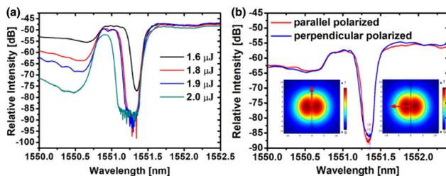
**Fig. 2.** (a) Resonant spectral transmission of first-order BGWs inscribed with different Bessel pulse energies. (b) Resonant spectral transmission of first order BGWs inscribed with pulse energy of  $1.6 \mu\text{J}$  upon injection with two orthogonal linear polarizations. The insets show the energy flux profiles for the parallel-polarized (left) and perpendicular-polarized (right) modes.
