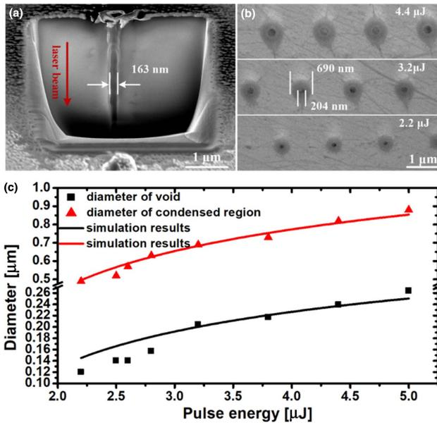
**Fig. 3.** (a) Longitudinal section of the grating void (2.8  $\mu\text{J}$ ) after material removal by FIB. (b) Cross sections of the post-polished grating voids induced by picosecond Bessel beam with different pulse energies. (c) Dependence of the voids' diameters and surrounding condensed region on pulse energies.
