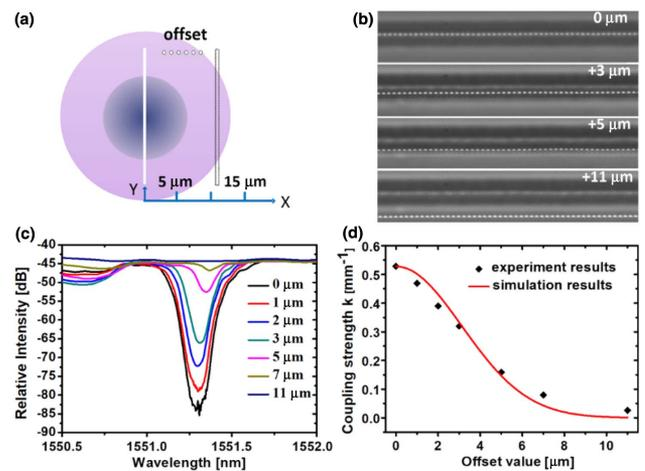
**Fig. 5.** Bessel voids were inserted into the waveguide with different offsets relative to the center of the waveguide's cross section. The pulse energy of the picosecond Bessel beam for inducing grating void was fixed at 2.2  $\mu\text{J}$ . (a) Diagram of the offset BGWs. (b) PCM top images of the spatially displaced BGWs. (c) Resonance spectra of third-order BGWs with different offset values. (d) Dependence of coupling strength on the offset value.
