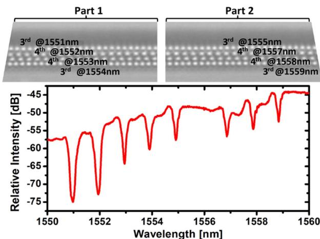
**Fig. 6.** BGW with multiple resonance peaks inscribed with Bessel laser pulses. Case in which eight third- and fourth-order gratings with different resonance peaks were inserted into the same waveguide in a parallel-serial-combined method. Both the lengths of Part 1 and Part 2 are 9 mm.
