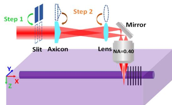
**Fig. 1.** Schematic fabrication setup for BGWs: the waveguide is first photoinscribed by using femtosecond Gaussian pulses in a slit shaping method, then the picosecond Bessel pulses are generated by using an insertable  $4f$  system with an axicon element to induce grating voids inside the waveguide along the  $x$ -axis direction.
