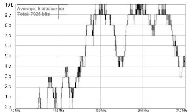
Fig. 5. Bits per carrier from the embedded PLC modem.
