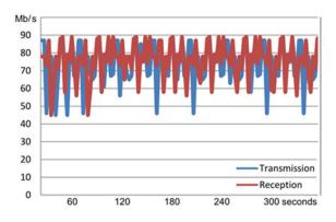
Fig. 11. TX and RX variation, frequency band 13 - 33 MHz.
