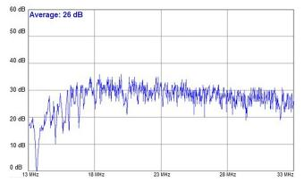
Fig. 8. SNR from the embedded PLC modem, freq. band 13 - 33 MHz.
