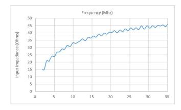
Fig. 3. Input impedance in PLC modem frequency operation band.
