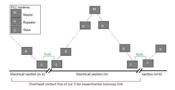
Fig. 13. V2I PLC network deployment topology.
