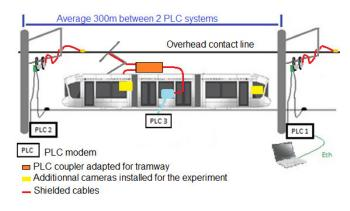
Fig. 1. Experimental installation of the tramway PLC link.
