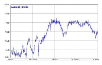
Fig. 4. SNR from the embedded PLC modem, freq band 4-34 MHz.
