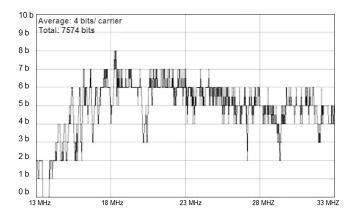
Fig. 9. Bits per carrier from the embedded PLC modem, sub freq. band 13 - 33 MHz.
