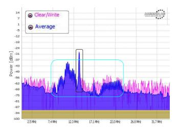
Fig. 2. Screen shot of the EM fields measured inside running tramway.
