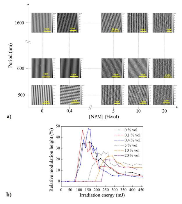
**Figure 3.** a) AFM topography images for structures with periods 1.6  $\mu$ m, 600 nm, 500 nm, and for particle concentrations in the 0–20%vol range. b) Relative modulation height versus the irradiation energy and MNP concentration, for structures with the period of 600 nm and initial thickness of 8 ± 5 nm.
