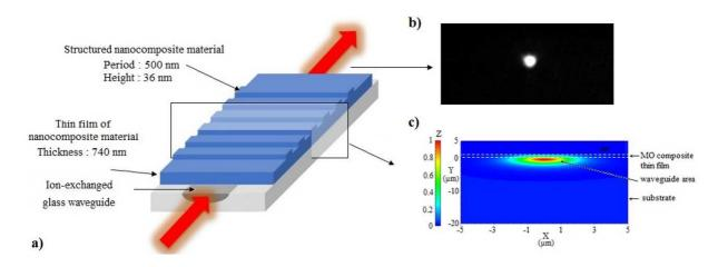
**Figure 5.** a) Schematic of the guiding sample prepared as a Bragg resonator on a waveguide. b) A photograph of the light beam exiting the guide. c) Simulation results of the guided mode field amplitude profile, performed using Optiwave BPM, for a 1- $\mu$ m-thick MO film on a waveguide.
