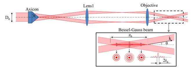
**Figure 9.** Schematic of the Bessel-Gaussian beam configuration, including an axicon and a standard 4f telescopic system (an achromatic lens and a microscope objective). The inset describes standard parameters of the Bessel beam with  $D_0$  is the incident Gaussian beam diameter,  $\alpha$  is the physical or base angle of the axicon,  $Z_b$  is the Bessel length,  $\theta$  is the half cone angle, k is the wave vector, and  $2r_b$  is the diameter of the beam central core.
