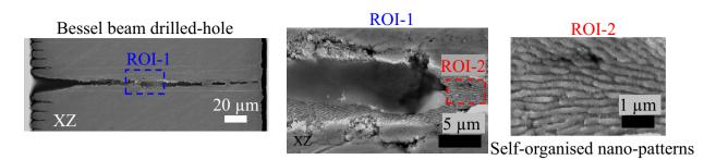
**Figure 6.** SEM cross-sectional image of the hole drilled through the 200  $\mu$ m steel plate by the Bessel beam at the laser fluence F = 5.15 J/cm<sup>2</sup> (Left); Blow-up images in the ROI-1 (Middle) and ROI-2 (Right), showing the self-organized nano-structures induced by the self-replication of the Bessel beam.
