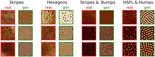
**Fig. 2** Comparison between real SEM images (red) and SH-generated images (green). SH generated images are able to reproduce a variety of patterns (e.g., stripes, hexagons, bumps, HSFL, humps) and scales [5]. Since the SH model is an isotropic model, global symmetries are only apparent (e.g., oriented stripes), whereas SEM images retain some measure of global symmetry from laser polarization.
