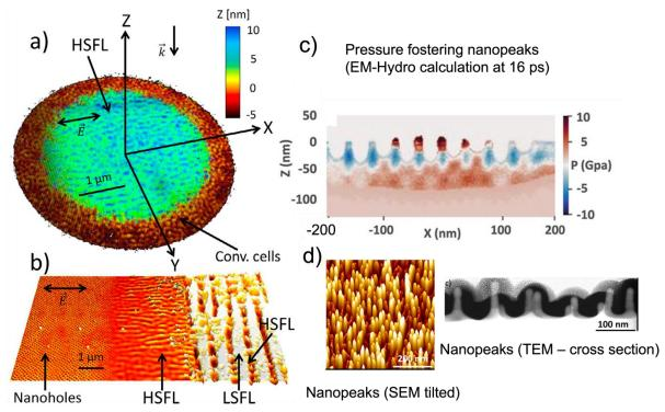
**Fig. 1** Comparison between EM-hydrodynamics simulations (a-c) with experimental SEM images (b-d) for nanocavity and HSFL formation conditions (a-b) and nanopeaks generation (c-d) upon ultrafast laser irradiation (100 fs duration). A double-pulse irradiation sequence (25 pulses) with crossed linear polarization has been used to generate the structures. The delay between sub-pulse and the local fluence regulate the kind of patterns.
