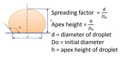
diameter is 2mm the static contact angle ( $\theta_e$ ) is 76° *at impact velocity of* 0.8 m/s
