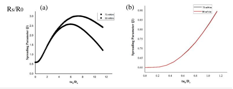
Spreading parameter on a plain (a) and on a triangular (b) Ti-6Al-4V surfaces at different surface tension.
