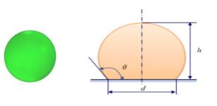
Diameter of droplet = 2 mm Impact velocity = 0.56 m/s Equili. Contact Angle = 106
