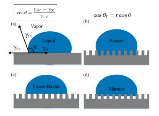
Wettability changes with surface relief, with surface/liquid/gas compositions, with droplet size and... Wettability changes with ...time!
