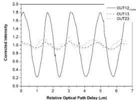
Fig. 3: Image of the monochromatic fringes of output peak 12 (OUT12<sub>CORR</sub>), together with residual fringes observed in OUT13 and OUT23.
