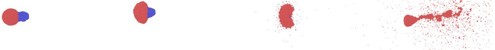
Simulations starts from Alloy AuCo NP, R=40 uc rapid heating above  $T_c$
