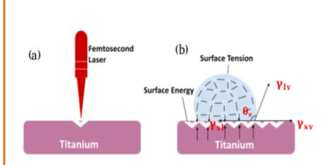
Fig 1. wettability of laser-treated titanium
